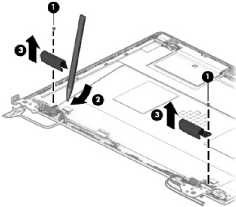
7. If it is necessary to replace the hinge brackets, remove the three Phillips M2.5×3.0 screws from the bottom of each hinge (1) and the Phillips M2.0×3.0 screw from the top of each hinge (2).
