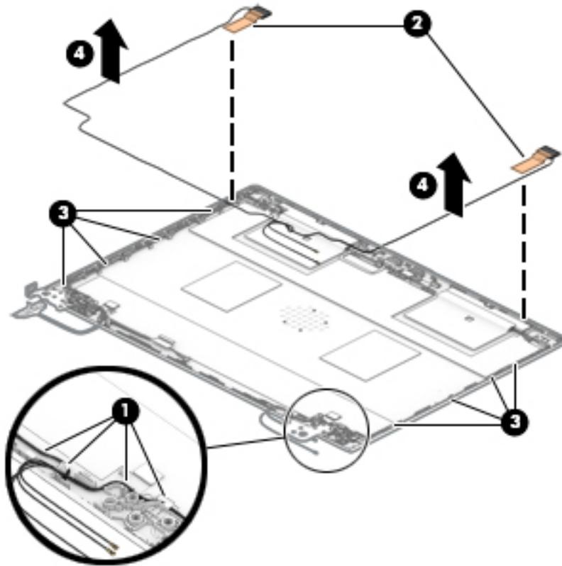
12. If it is necessary to replace the WWAN antenna cables, note the proper cable routing through the right hinge (1).
