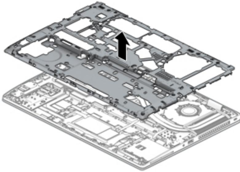
Reverse this procedure to install the internal frame.
