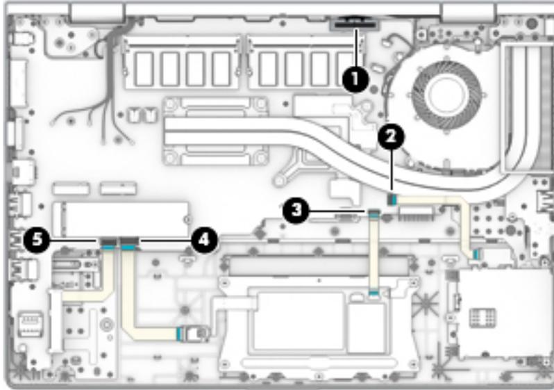
5. Remove the Phillips M2.0×3.0 screw (1), and then loosen captive Phillips screw (2) on the fan.
