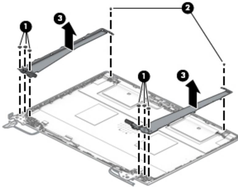
9. If it is necessary to replace the WLAN antenna cables, note the proper cable routing through the right hinge (1).
