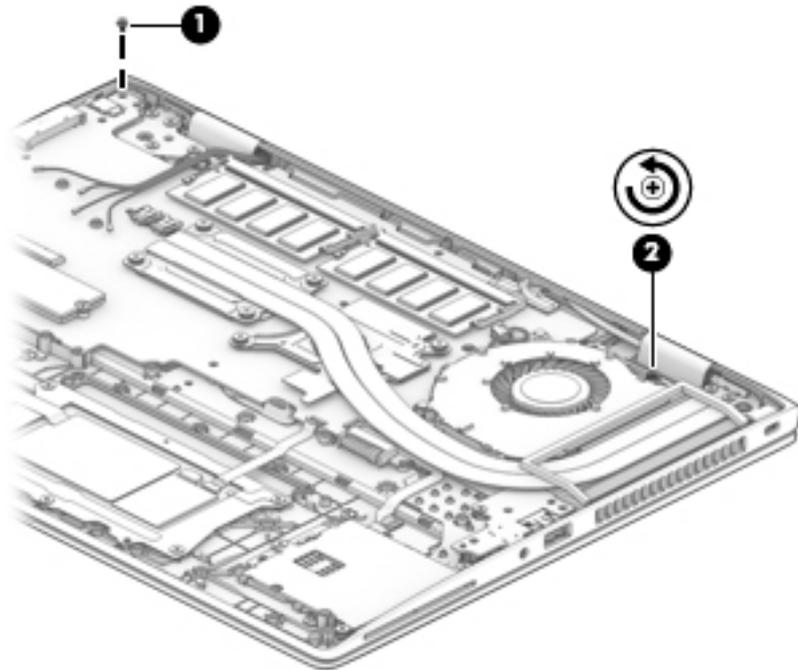
6. Lift the right side of the system board **(1)**, and then pull it to the right to remove it from the computer **(2)**.
