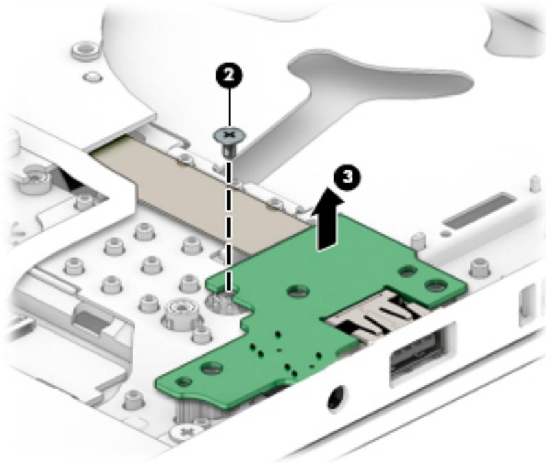
Reverse this procedure to replace the USB board.
