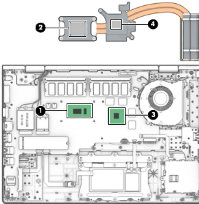
Reverse this procedure to install the heat sink assembly.
