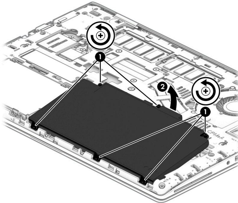
Reverse this procedure to install the battery.
