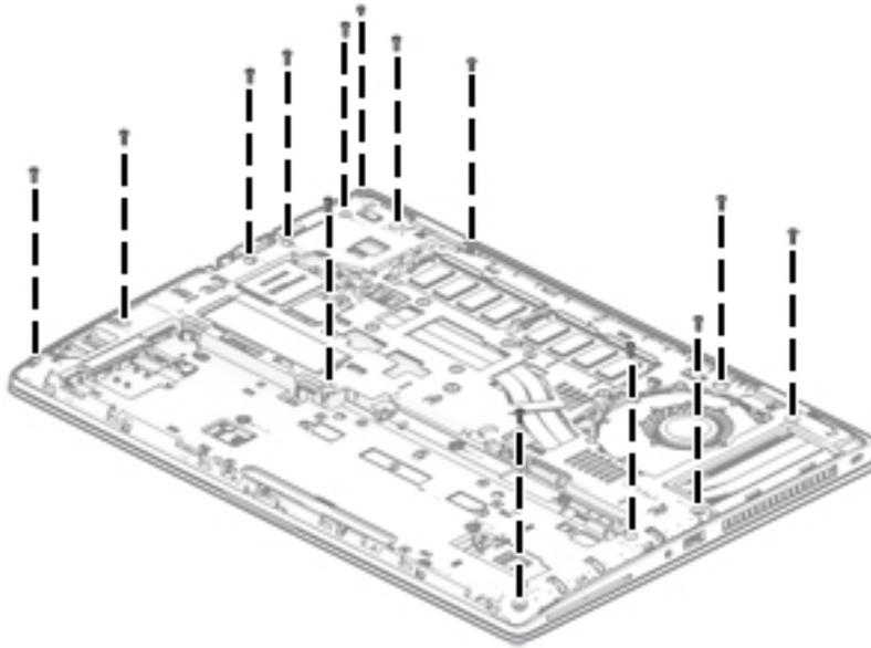
3. Remove the following screws that secure the frame to the computer:
