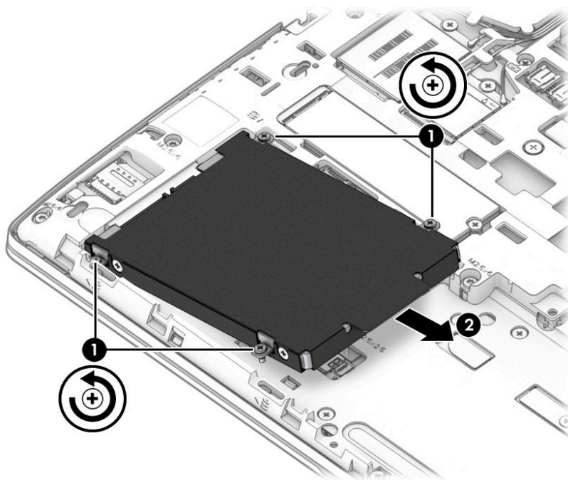
3. If it is necessary to disassemble the hard drive, remove the four Phillips M3.0×3.0 screws (1), and then slide the drive out of the drive cover (2).
